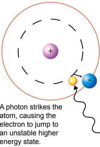
A photon strikes the atom, causing the electron to jump to an unstable higher energy state.
