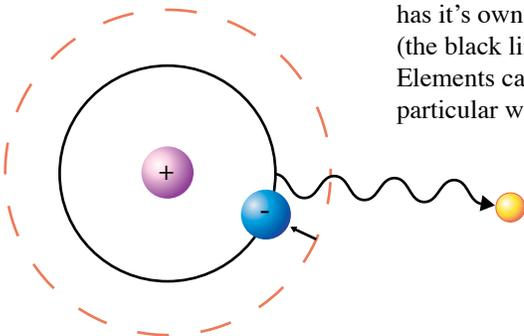
The electron loses the extra energy and jumps back to a lower energy state; the extra energy lost is emitted by the atom as a photon.
